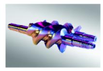
energy savings of the Delta Hybrid and its competitors. When passing the inlet port, the volute of the female rotor fills with air. As the rotors twist, the matching lobe of the male rotor reduces the volume of the volute, compressing the air. When the volute reaches the discharge port, the air is at the discharge pressure of the system. For the Delta Hybrid, this occurs four times for each revolution of the shaft, since there are four volutes.
